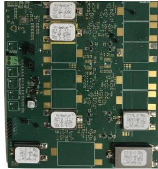
Power management board
