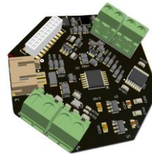
Sensing board- air temperature, humidity and soil temperature
